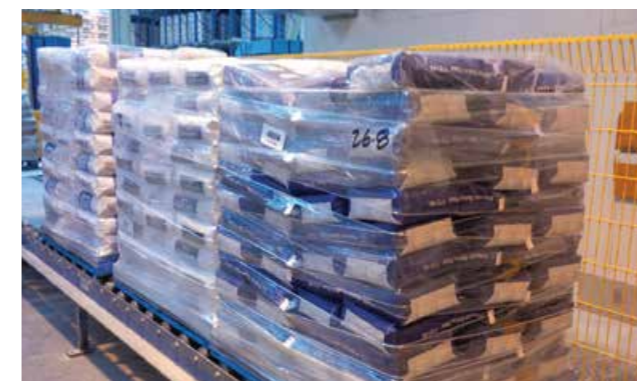
Banding increases airflow on hot products to help eliminate condensation
